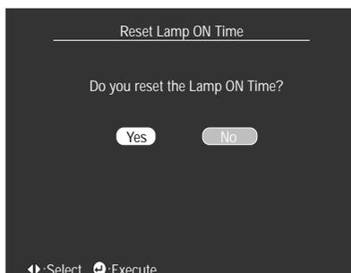
2. Use the left arrow button (control panel) or press left on the **Enter** button (remote control) to select **Yes**.
